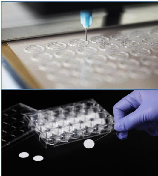
ST1's innovative 3D bioprinting technique solves the problem of conventional nanofibers and enhances mobility of the nanofibers. Users can select the thickness, the orientation of nanofibers and frame pattern on the surface of nanofibers according to the intended use.
